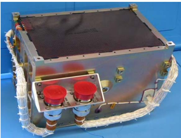
Figure 9: 28V, 26Ah Mars Science Laboratory Qualification Battery.
